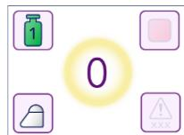
If the DEFINITY® vial does not shake for the full 45 second duration or at the acceptable rate, activation is not considered successful and the vial must not be used. An error message will be displayed and an audible alarm will sound to alert the user. Refer to page 9 for a list of error messages and the conditions they indicate.
