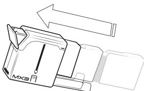
**5** Tilt Dispenser Up, Allowing Test Strips to Slide into Dispenser
