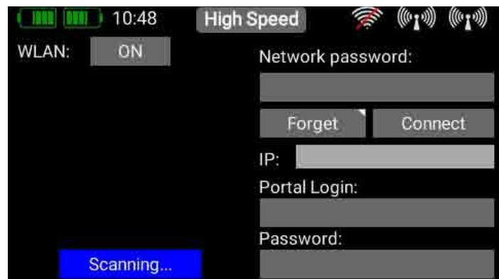
The WiFi module in the transmitter immediately searches for all WLAN hotspots which are in range.
