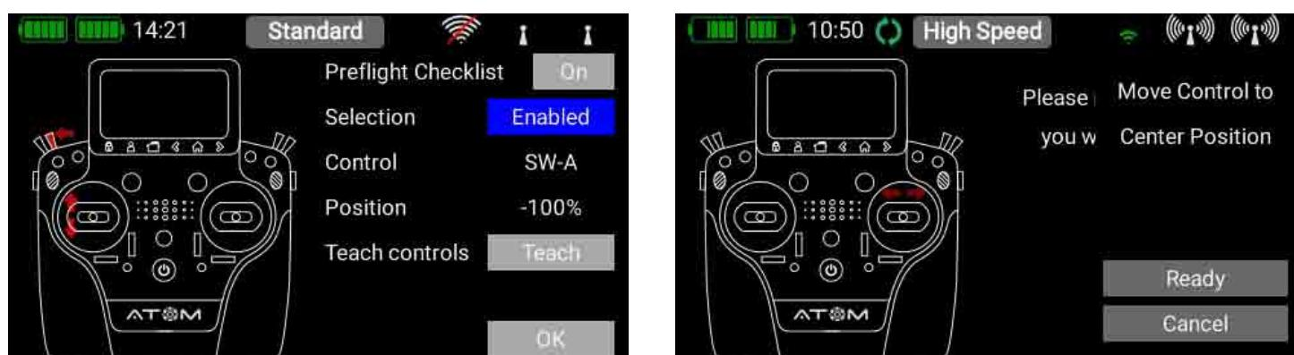
If you have installed a proportional control or a 3-position switch, you also need to move the transmitter control to the center. Touch Finished to complete the process. The **Direct** button can be used to reverse the transmitter control's direction of operation.
