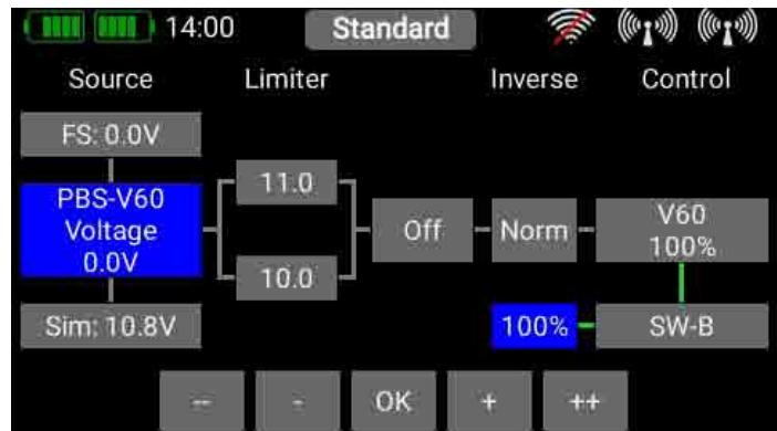
To conclude our example, you can now see how the telemetry control is set in such a way that motor power is reduced by 50% when battery voltage falls to 11.0V.
