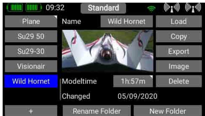
To create a new model, briefly touch the + button at the bottom of the screen. Assign a name to your model, and confirm your choice with OK. You will now see the Select screen for the model type. At this point you can select the appropriate model type, with the additional options of delta wing and V-tail.
