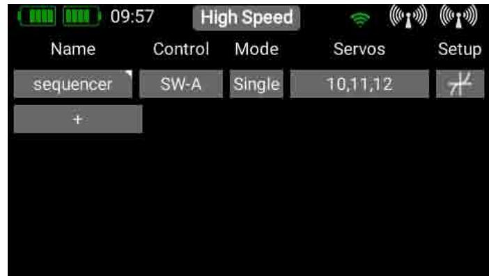
At the Overview screen press **Setup** to set the travel points. You will see the next screen display shown here. The first servo is marked, and the sequence **Forward** and **Reverse** is displayed. The standard run time is 6.0 seconds, and the two travel points are set at  $\pm 20\%$ .
