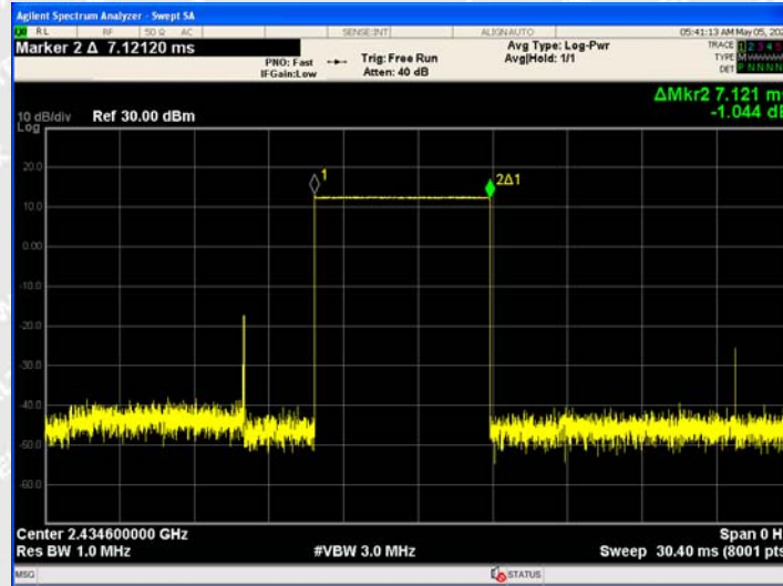
Chart of burst length in 30ms (trigger offset-0.5ms)
