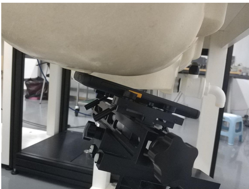
Picture 6: Right Hand Tilt 15° Position
