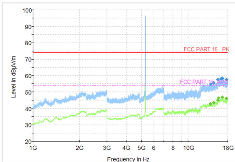
Fig. 87 Transmitter Spurious Emission (802.11n-HT40, CH62 5310MHz)
