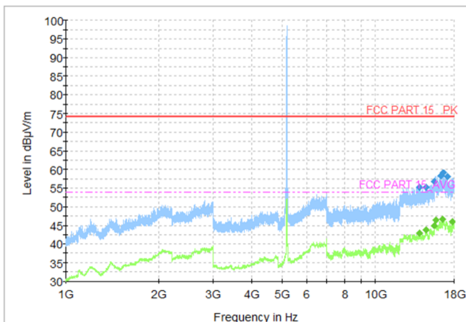
Fig. 84 Transmitter Spurious Emission (802.11n-HT40, CH38 5190MHz)
