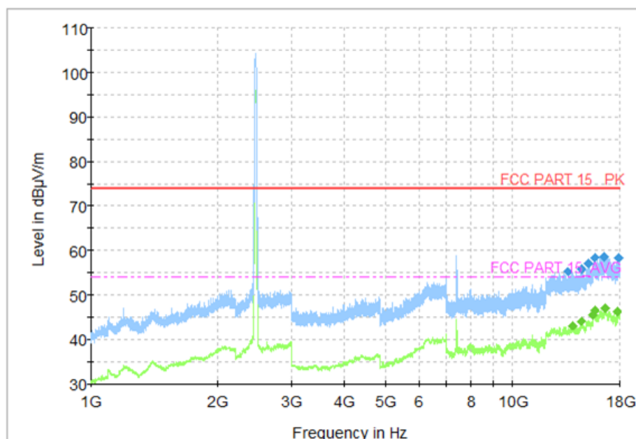
Fig.57 Radiated Spurious Emission (802.11n HT20, CH11, 1 GHz-18 GHz)
