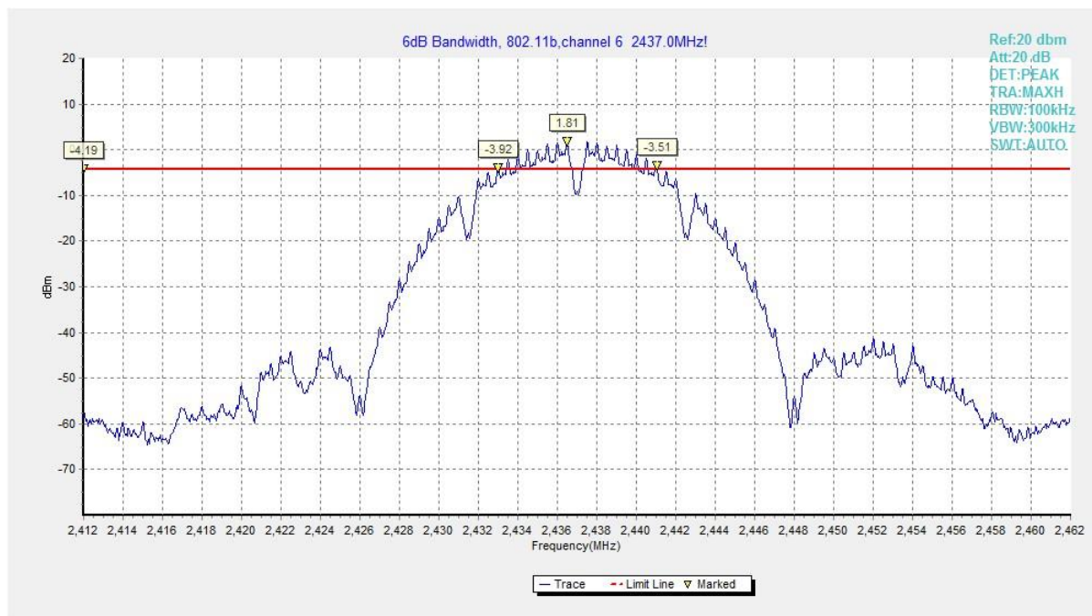
Fig.14 6dB Bandwidth (802.11b, CH 6)
