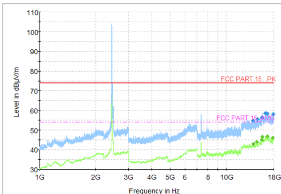
Fig.62 Radiated Spurious Emission (802.11n HT40, CH9, 1 GHz-18 GHz)
