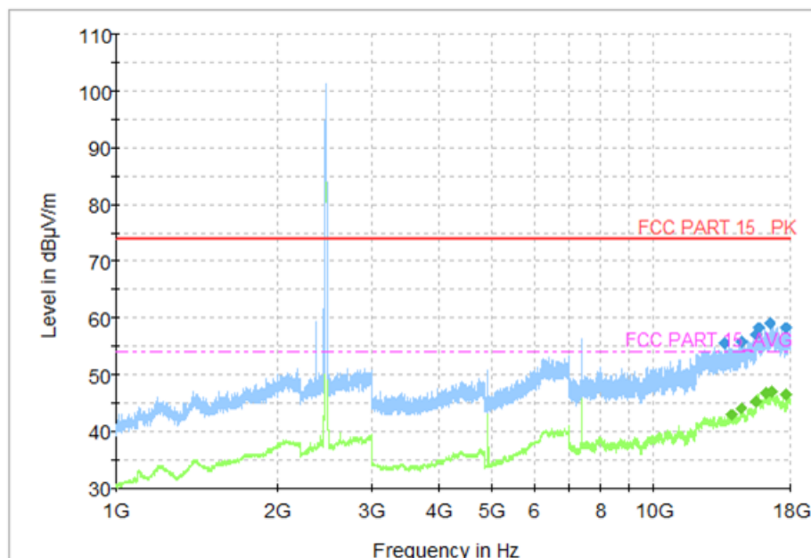
Fig.47 Radiated Spurious Emission (802.11b, CH11, 1 GHz-18GHz)
