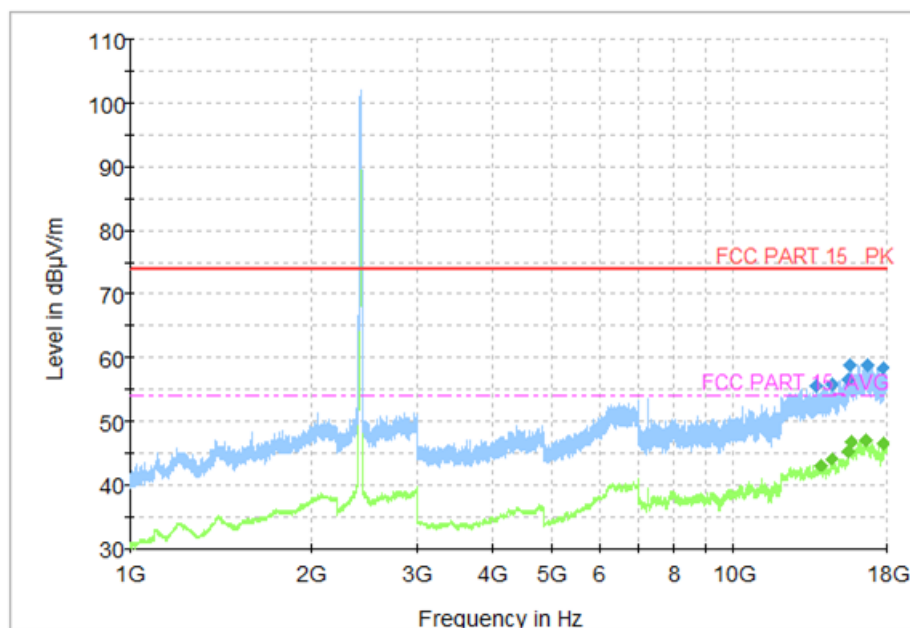
Fig.50 Radiated Spurious Emission (802.11g, CH1, 1 GHz-18 GHz)
