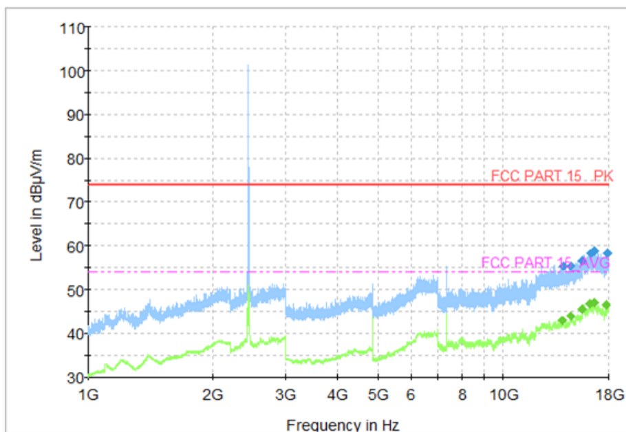
Fig.46 Radiated Spurious Emission (802.11b, CH6, 1 GHz-18GHz)
