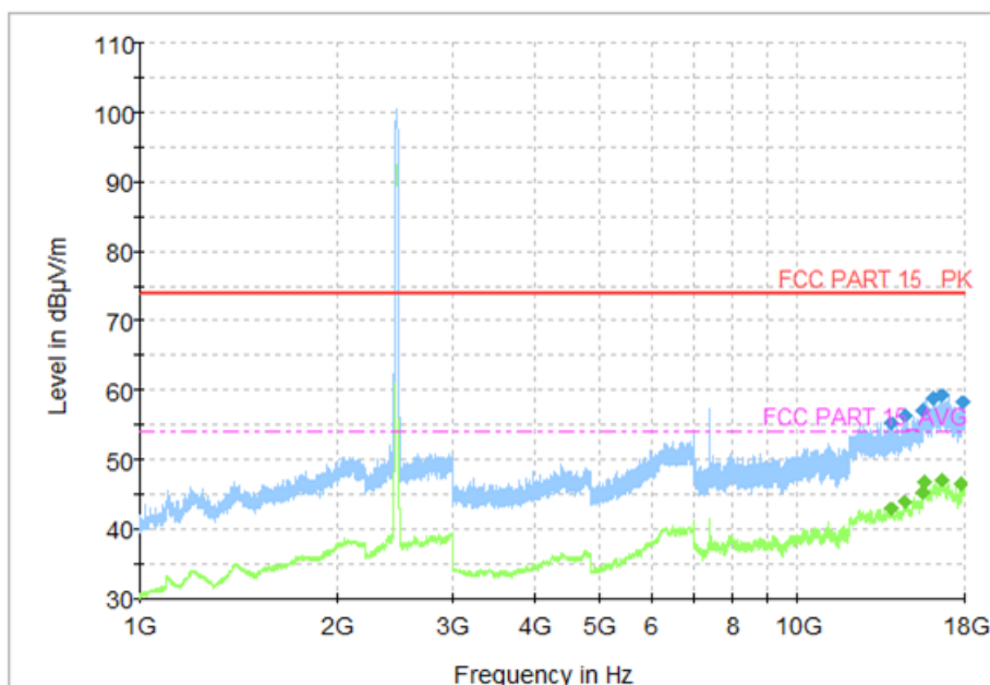
Fig.52 Radiated Spurious Emission (802.11g, CH11, 1 GHz-18 GHz)
