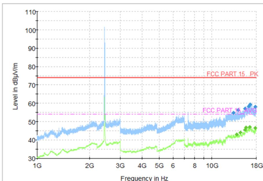
Fig.51 Radiated Spurious Emission (802.11g, CH6, 1 GHz-18 GHz)
