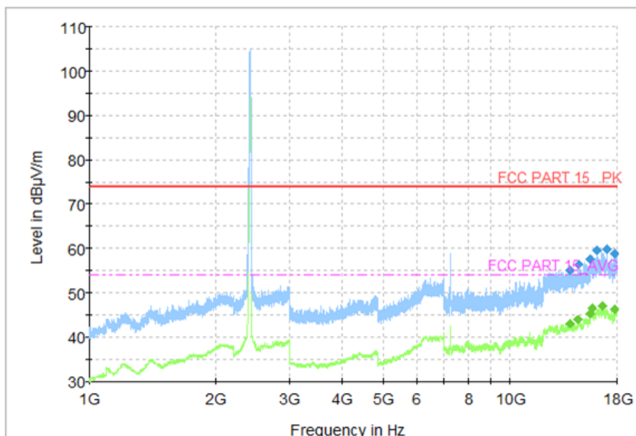
Fig.55 Radiated Spurious Emission (802.11n HT20, CH1, 1 GHz-18 GHz)
