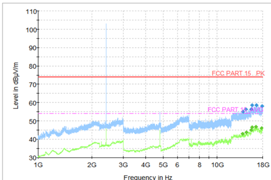
Fig. 52 Radiated Spurious Emission (8DPSK, Ch0, 1 GHz ~18 GHz)
