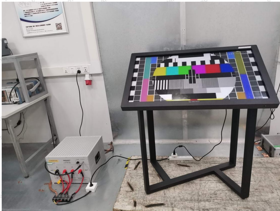
Photo of Conducted Emission Measurement
