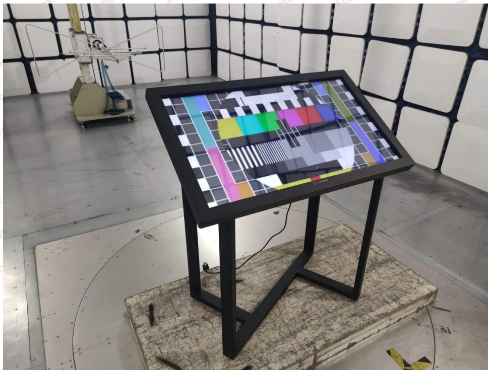
Photo of Radiation Emission Test
