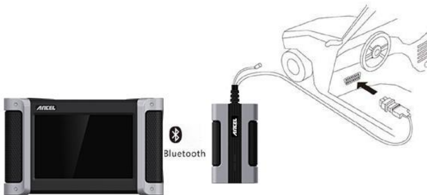
Figure 3.2-2 Connection of non-OBD-II port
