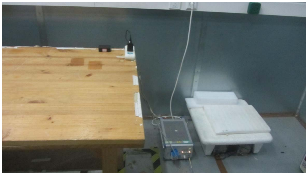
Picture 3 Conducted Emission Test Setup
