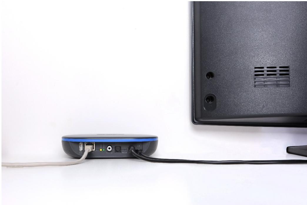
3. Use the microUSB cable to connect CloviFi to the TV's USB port or to the included power supply.
