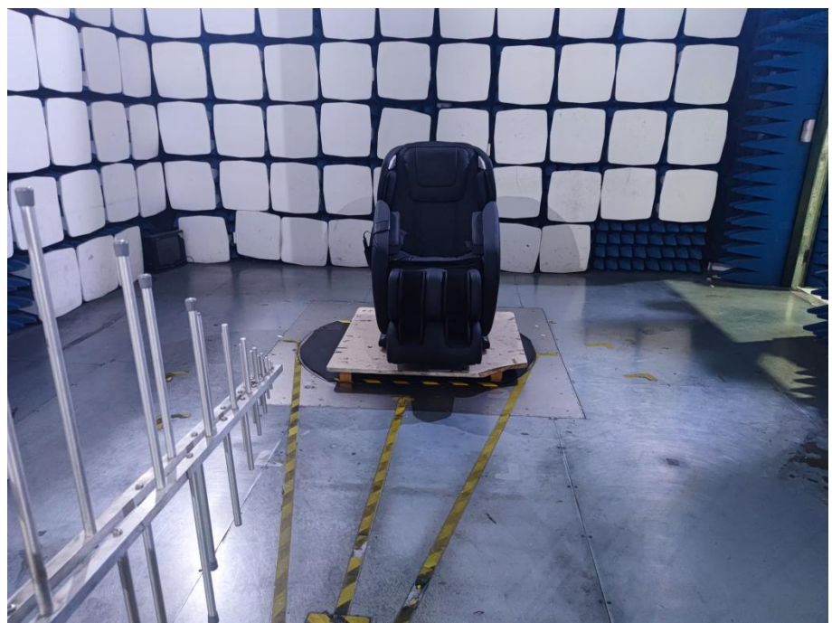
Radiation Emission Test Setup (30MHz to 1GHz)
