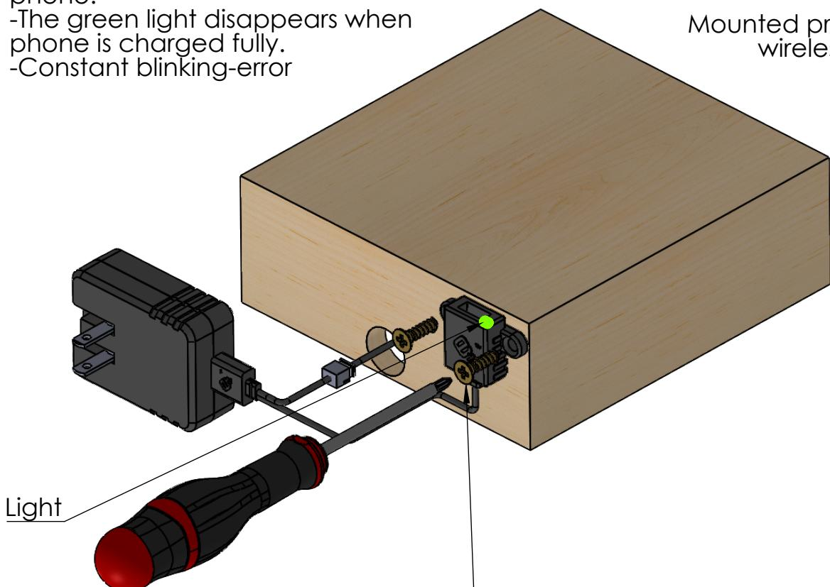
Screw in the USB HUB using a Philips screwdriver, using the screws provided
