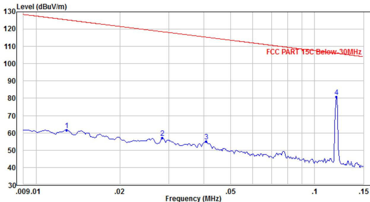
**Radiated Emission Test Data (150 KHz ~ 30 MHz):**
