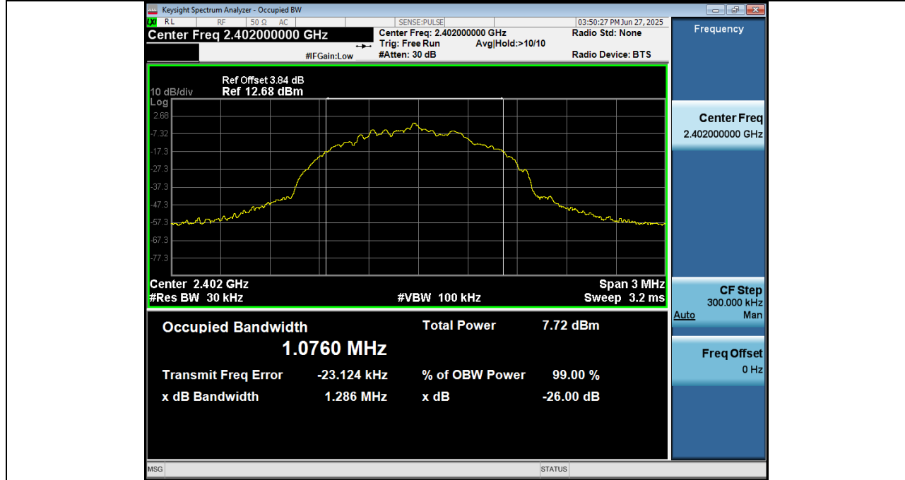
99% Occupied Bandwidth NVNT ANT1 1Mbps 2402
