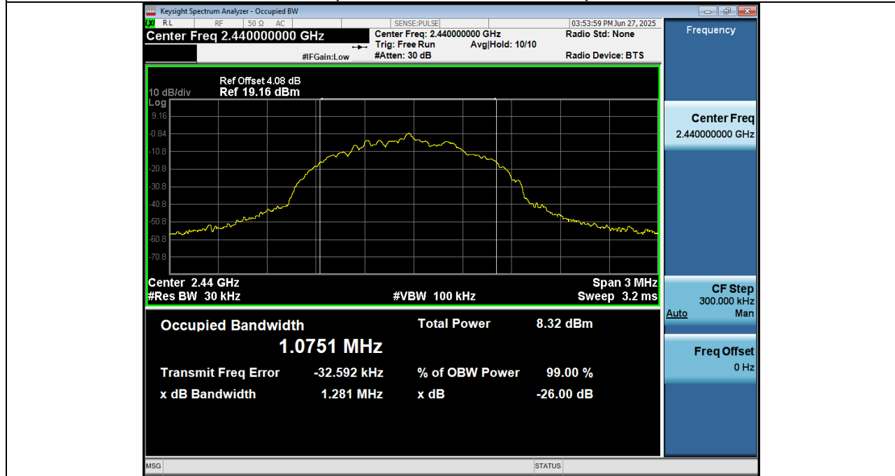
99% Occupied Bandwidth NVNT ANT1 1Mbps 2440
