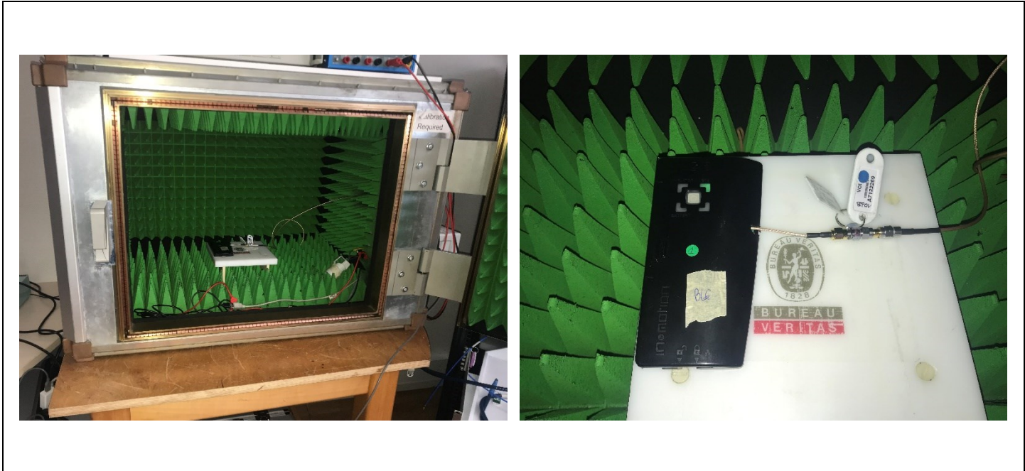
Photograph for Unwanted Emission into non-restricted frequency bands at the band edge
