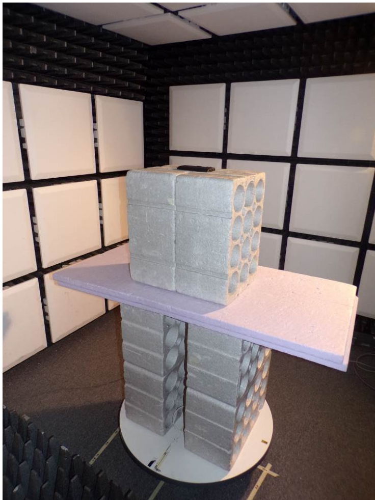
FAC setup (1GHz-25GHz / 3m)
