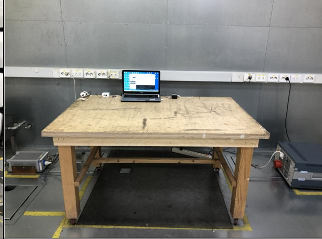
A photograph of a conducted emissions test setup. A wooden table is positioned in a room with grey walls. A laptop is placed on the table, connected to various test equipment. A power strip with multiple outlets is visible on the wall behind the table. |
