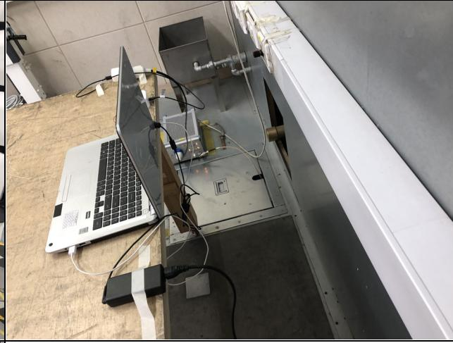
A close-up photograph of the conducted emissions test equipment. A laptop is connected to a signal generator and a spectrum analyzer. The equipment is placed on a wooden table next to a metal cabinet.                                                    |
