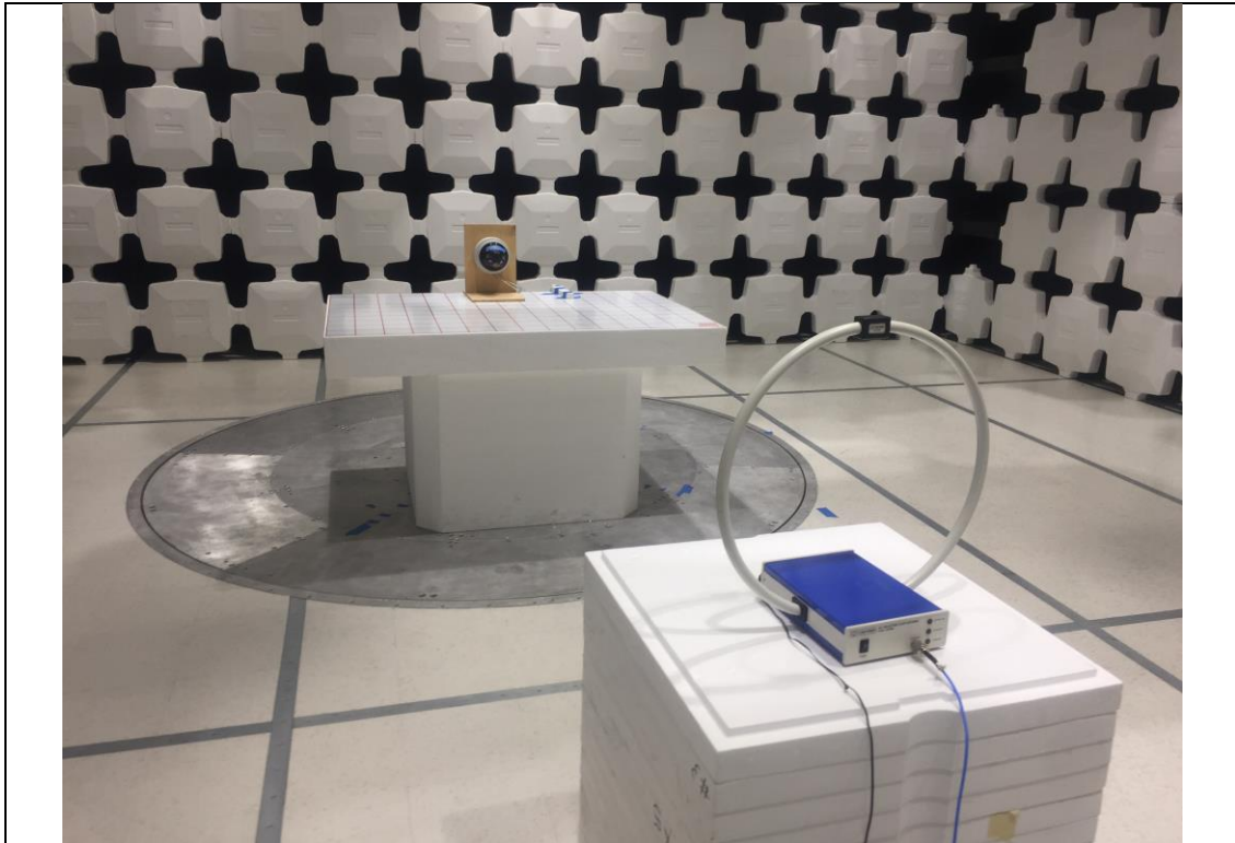
Radiated Emissions Below 30MHz setup – Front
