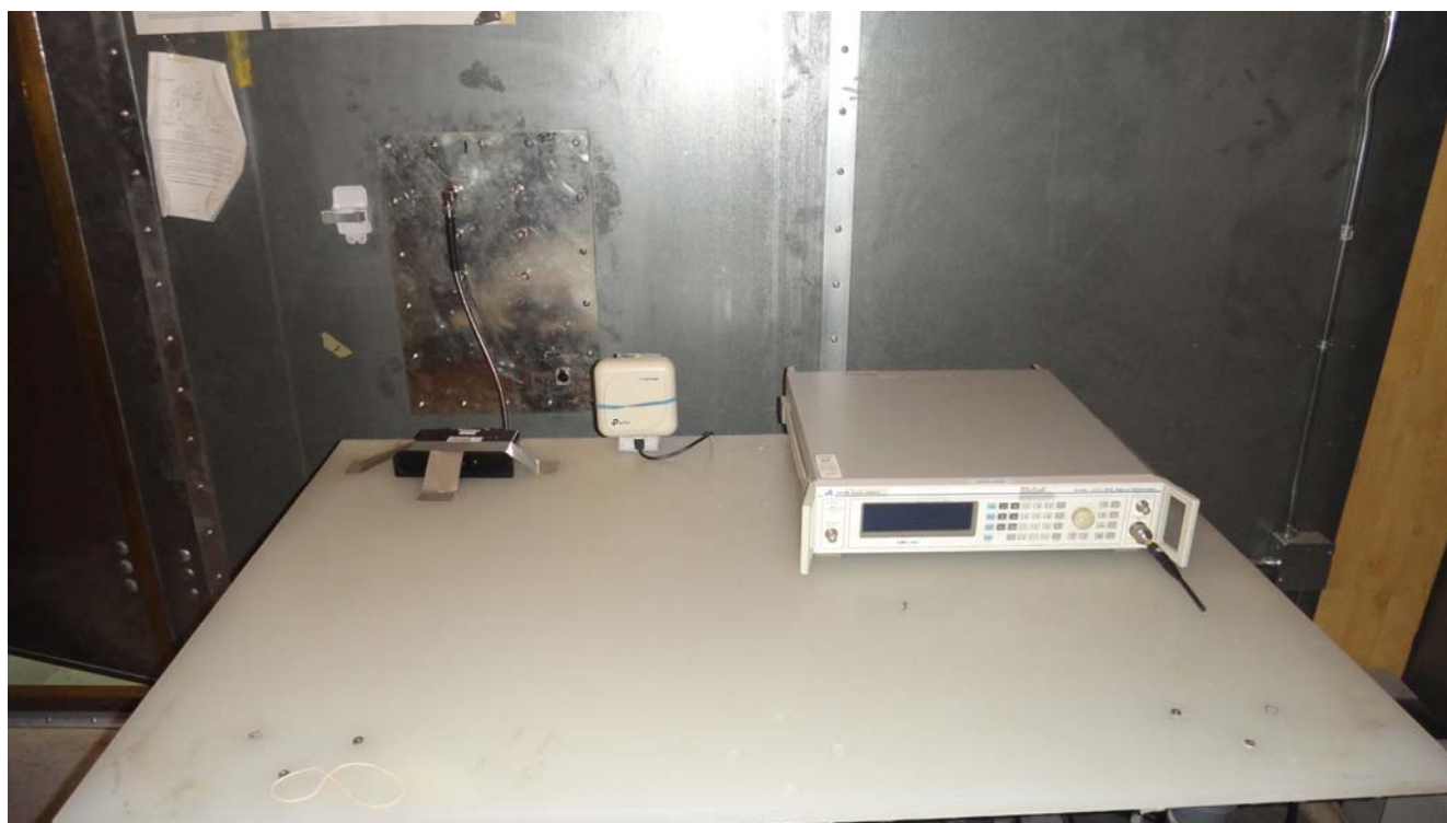
Power Line Conducted Emissions
