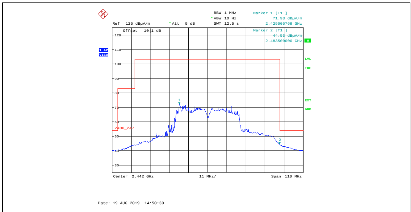
Plot 5.4.4.2.5.48. Band-Edge RF Radiated Emissions at 3 m, Horizontal Polarization, Average 802.11n HT40, 400 ns, MCS 7, 64-QAM 5/6 150.0Mbps, Power Setting 18, Channel 7, 2442 MHz
