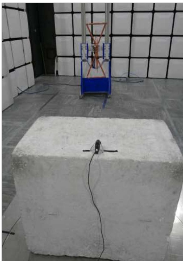
Figure 26 - Test Setup - 30 MHz to 1 GHz - Z Orientation
