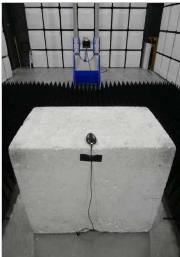
Figure 27 - Test Setup - 1 GHz to 13 GHz - X Orientation
