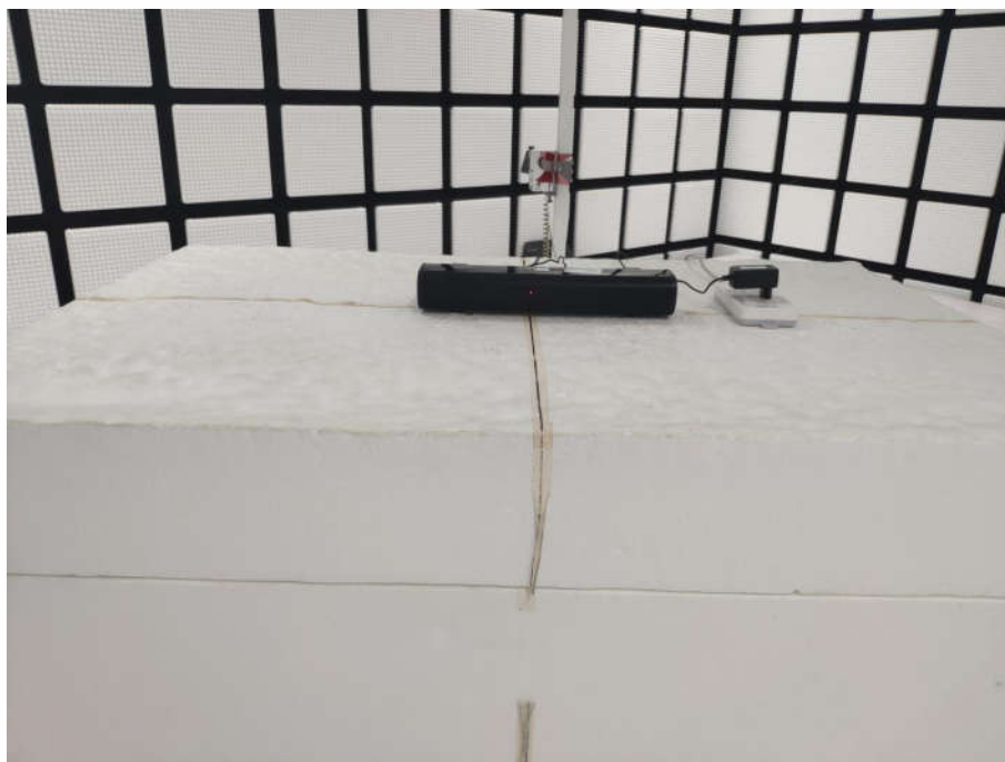
Radiated spurious emission Test Setup-3(Above 1GHz)
