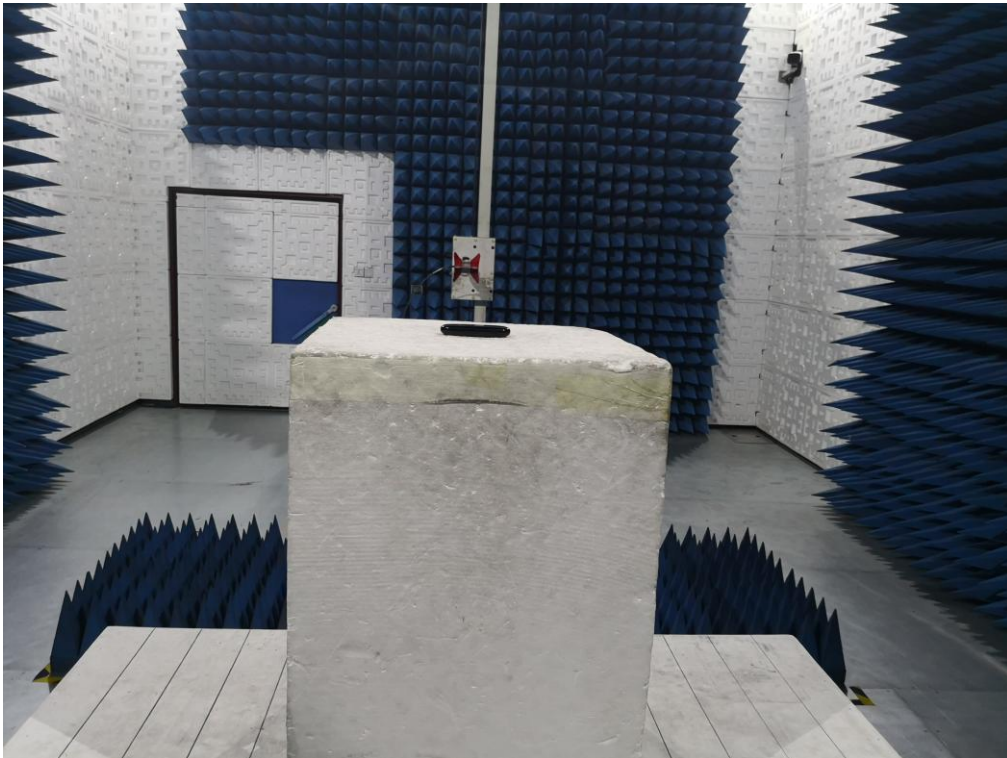
RADIATED EMISSION TEST SETUP ABOVE 1GHZ
