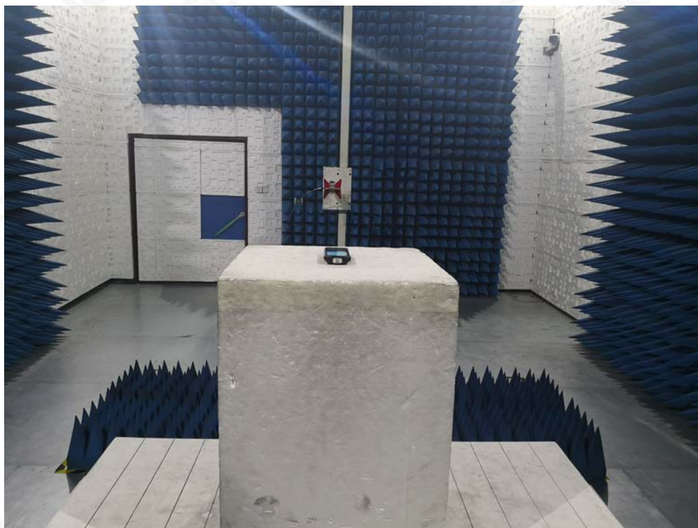
RADIATED EMISSION TEST SETUP ABOVE 1GHZ
