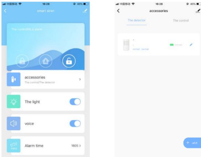
③ Click "OK" → smart siren light keep on → accessories send signals → smart siren light flash 3 times, adding is successful.
