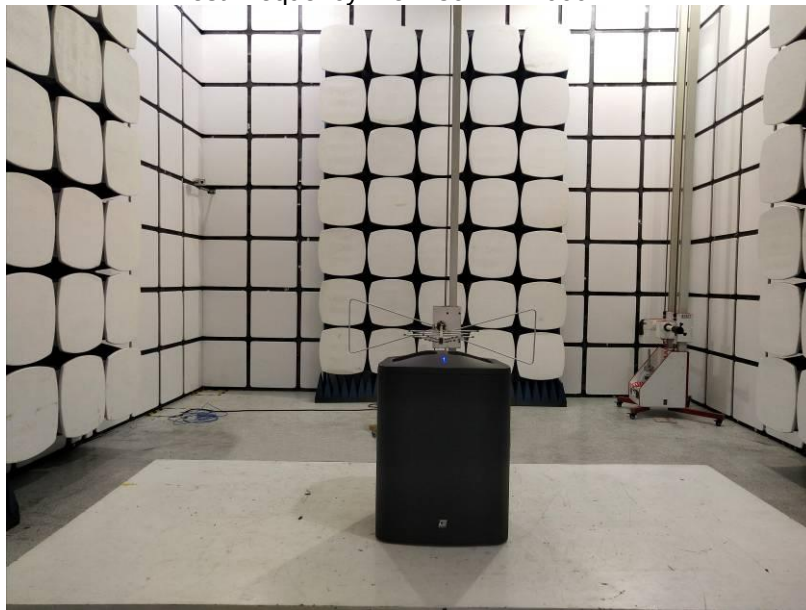
Radiated Spurious Emissions Test Frequency From 30MHz-1000MHz
