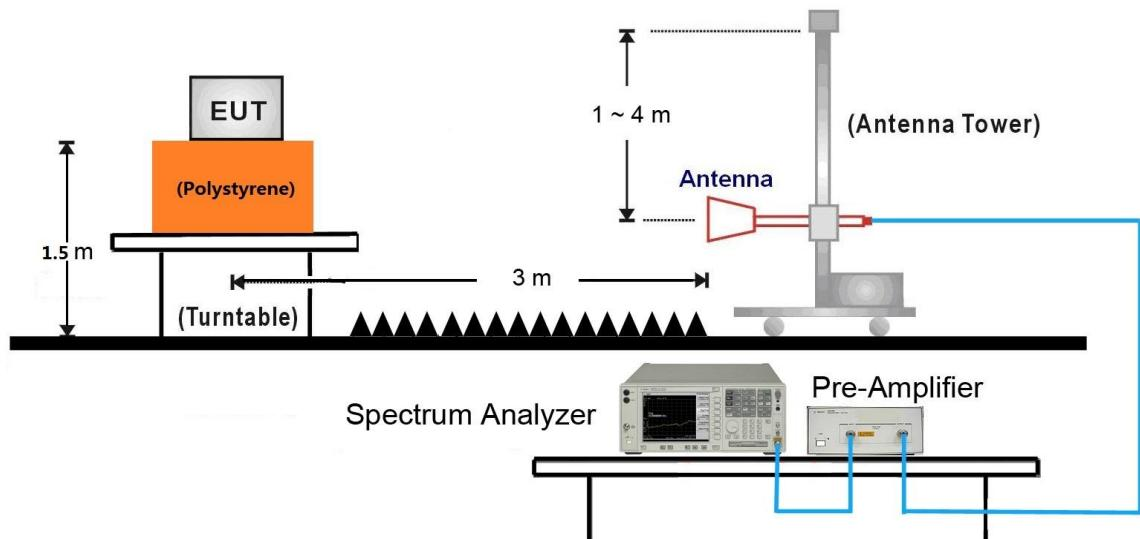
18GHz ~25GHz Test Setup:
