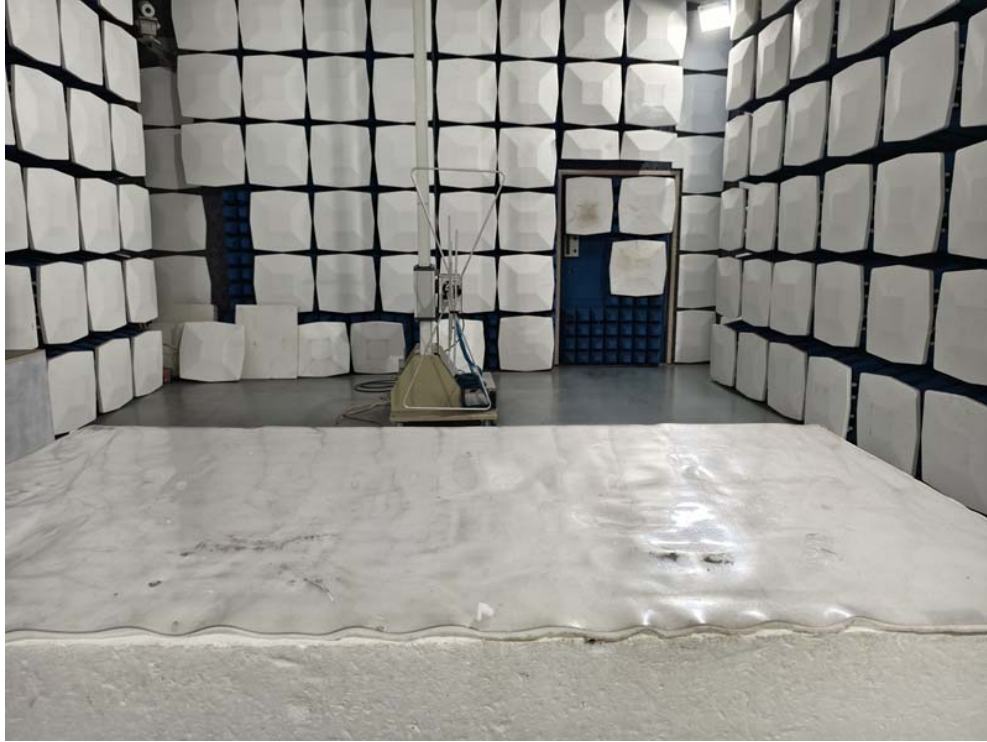
Radiated Emission Test Setup:
