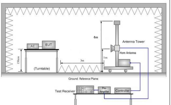
A technical diagram of an antenna test setup. It shows a 'Turntable' with an 'AE' (Antenna Equipment) and an 'EUT' (Equipment Under Test) on top. The turntable is 1.50m high. The distance between the turntable and an 'Antenna Tower' is 3m. The distance between the turntable and a 'Horn Antenna' is 4m. The 'Horn Antenna' is 1m high. The entire setup is on a 'Ground Reference Plane'. Below the turntable, a 'Test Receiver' is connected to a 'Pre-Amplifier' and a 'Controller'. |  |
