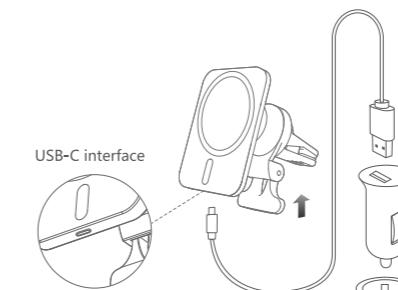
① Connect one end of the USB-C interface of the USB cable to the magnetic wireless charging USB-C interface.
