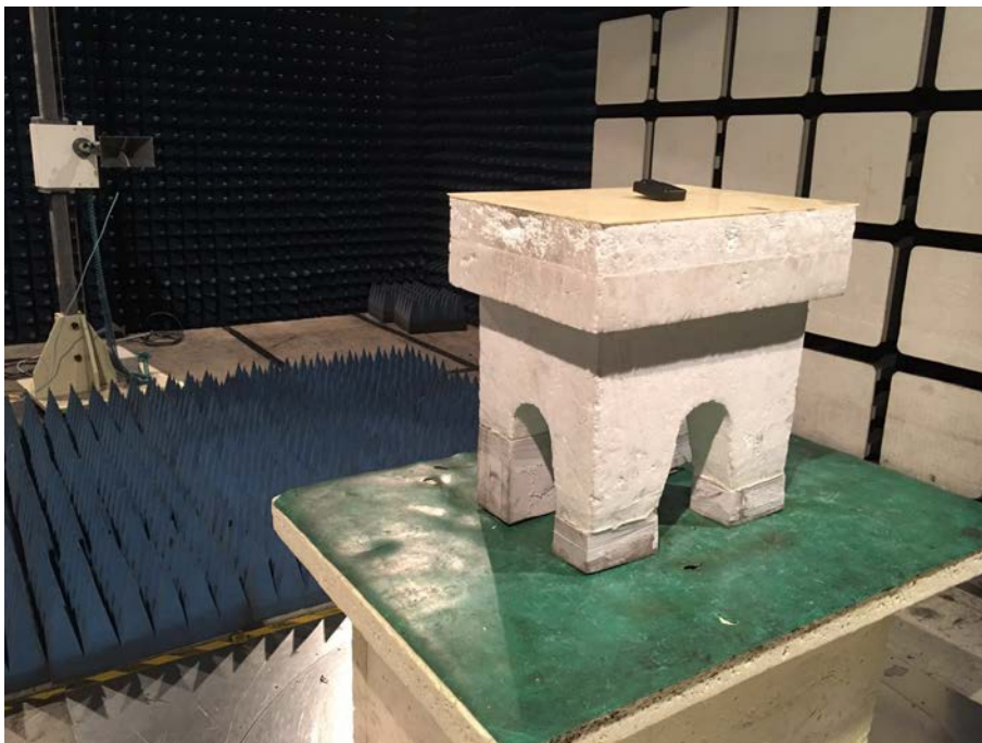
Spurious Emission Test Setup (Above 1GHz)
