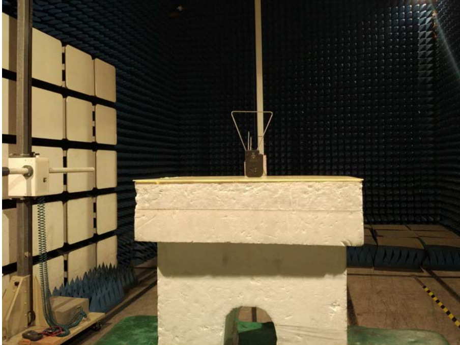
Spurious Emission Test Setup (Below 1GHz)
