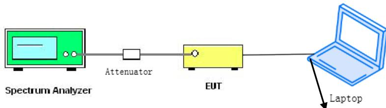
The EUT (Equipment under the test) is coupled to the Spectrum analyzer; the RF load attached to the EUT antenna terminal is 50Ohm; the path loss as the factor is calibrated to correct the reading, all test result in Spectrum analyzer.
