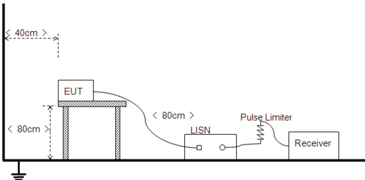
The Table-top EUT was placed upon a non-metallic table 0.8m above the horizontal metal reference ground plane. EUT was connected to LISN and LISN was connected to reference Ground Plane. EUT was 80cm from LISN. The set-up and test methods were according to ANSI C63.10: 2013.
