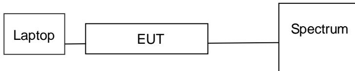
Note: 1. The EUT was used fully-charged battery programmed to be in continuously transmitting mode and the transmit duty cycle is not less than 98%.
