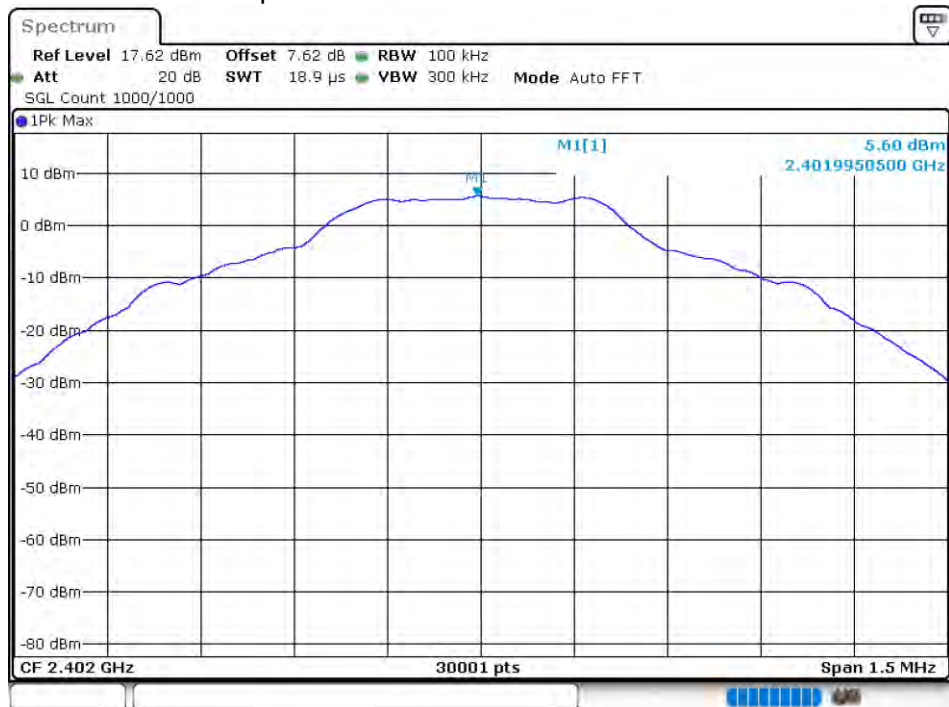
Tx. Spurious NVNT 1-DH5 2402MHz Ant1 Ref
