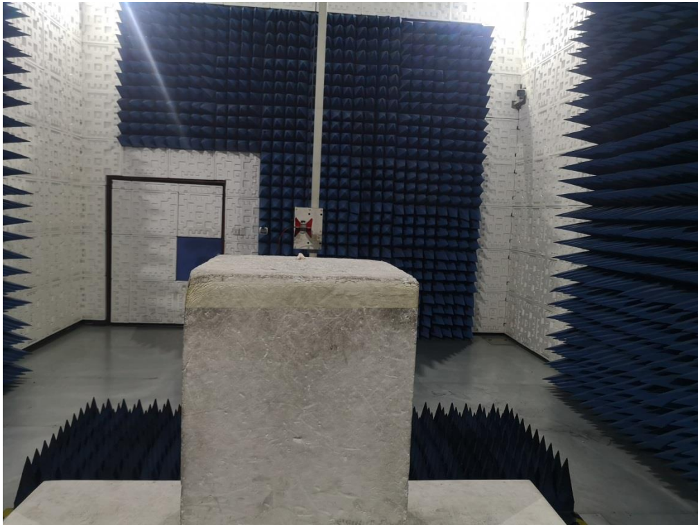
RADIATED EMISSION TEST SETUP ABOVE 1GHz
