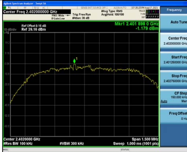
8DPSK on Channel 00
