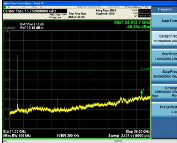
8DPSK on Channel 39
