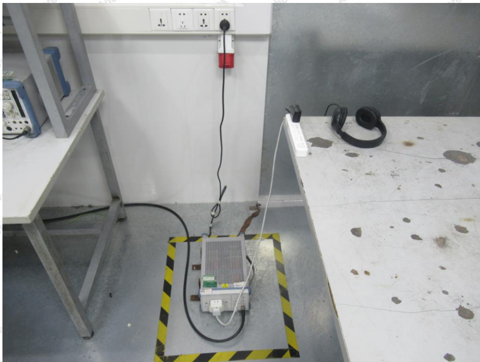
Photo of Conducted Emission Measurement
