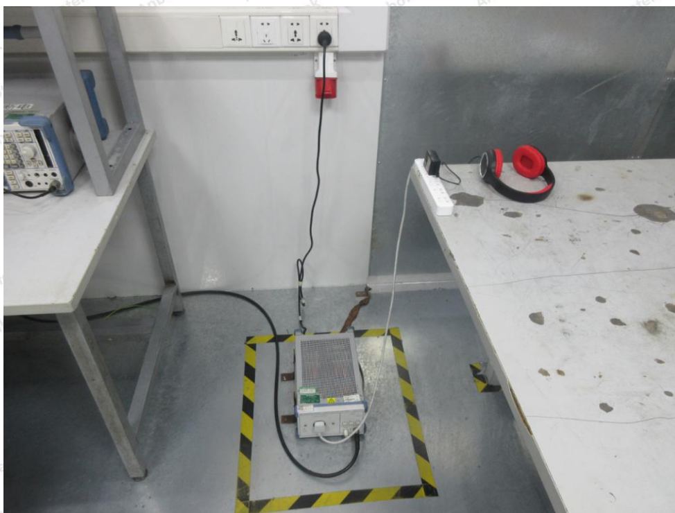
Photo of Conducted Emission Measurement
