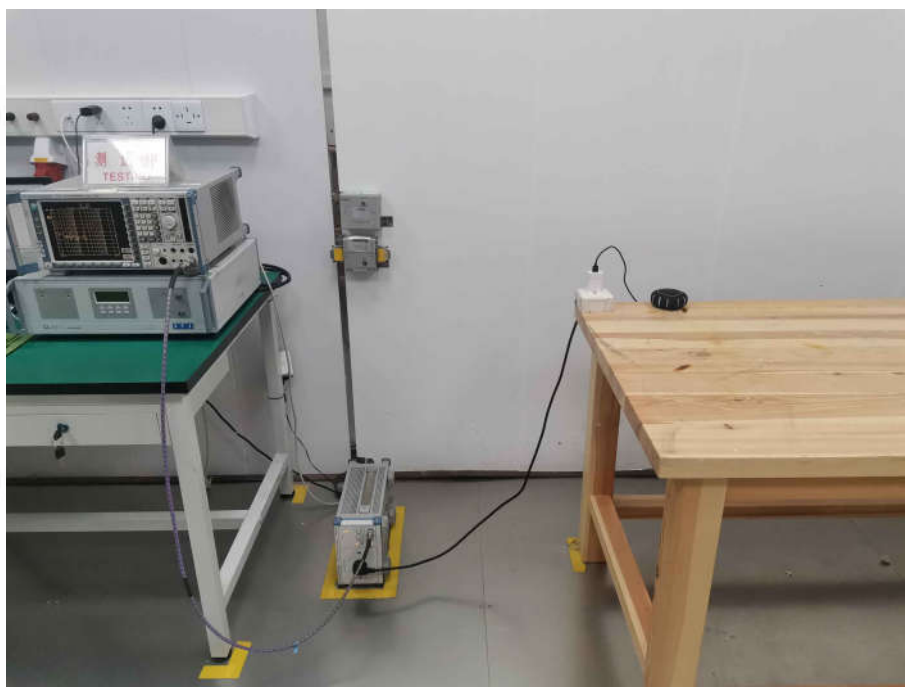
Conducted Emissions Test Setup
