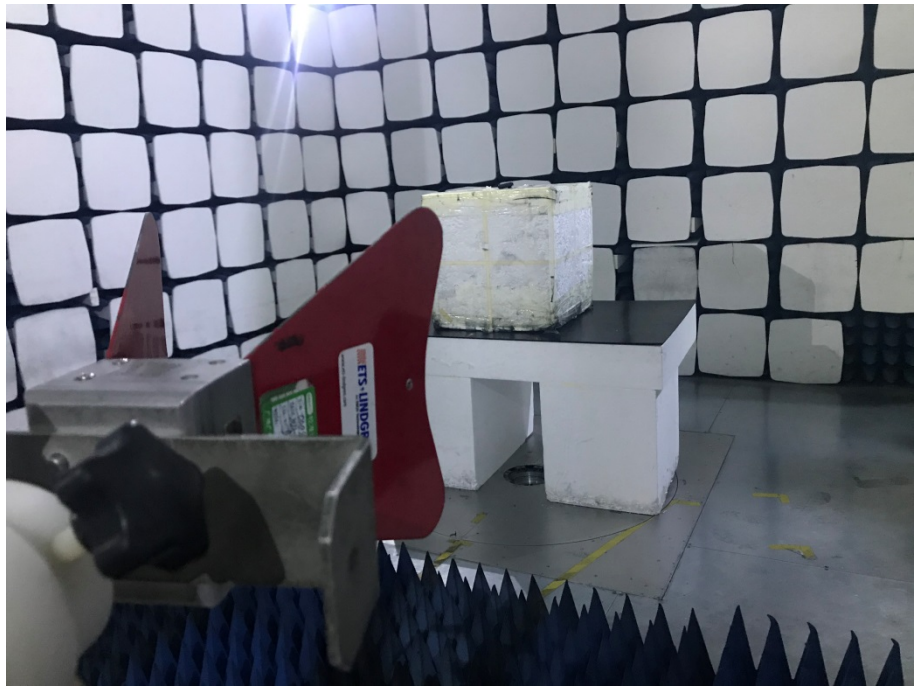
Radiation Emission Test Setup (1GHz to 18GHz)
