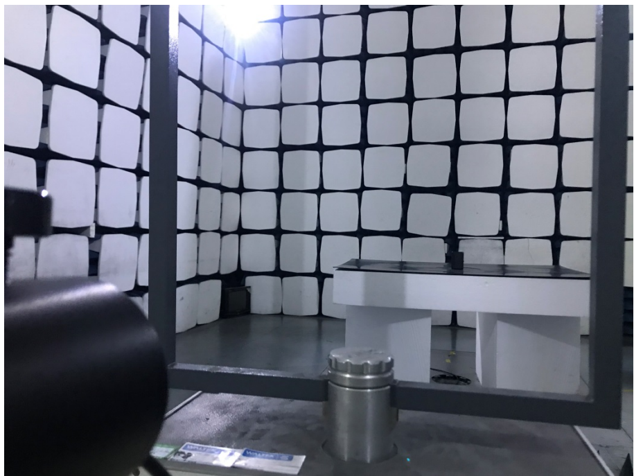
Radiation Emission Test Setup (Below 30MHz)
