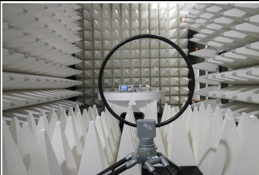
Radiated test setup below 30 MHz
