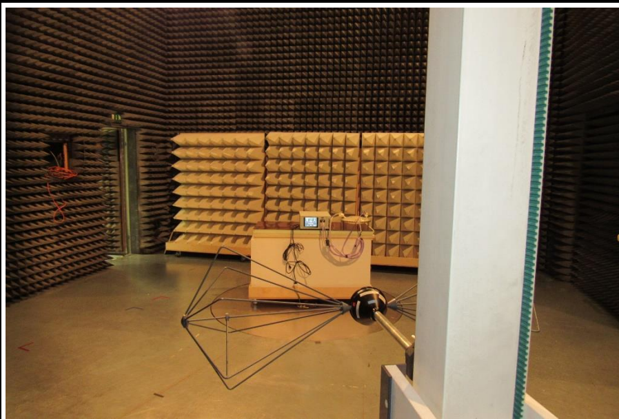
Radiated test setup view above 30 MHz - EUT hor
