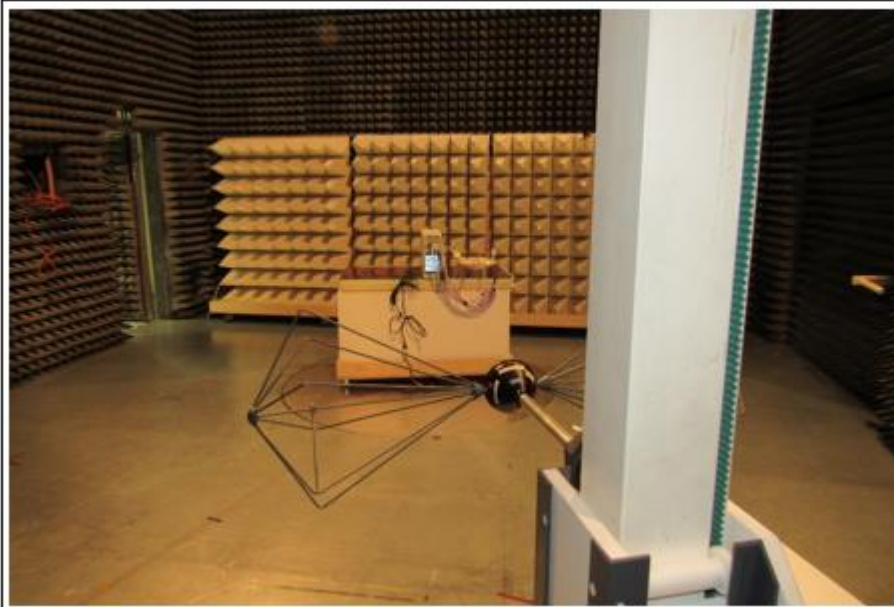
Radiated test setup view above 30 MHz - EUT ver
