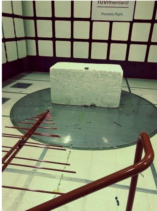
Figure 4 - Radiated Emissions Test Setup 30 - 1000 MHz - Front
