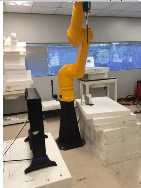
Figure 34 – Power source angle: 45° Client angle:-45° scan closest to WPT Source - Horizontal plane
