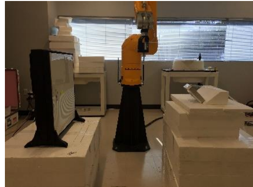
Figure 24 - Test setup: Scenario 5 Power client angled 45°
