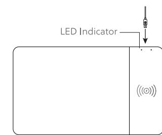
**3.** Place your Qi-standard device on the wireless charging mousepad area to start wireless charging. LED lights will start pulsing, indicating the device is charging.
