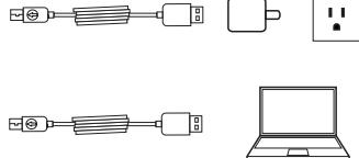
**2.** Insert the small end of the USB charging cable into the Micro USB port of the wireless charging mousepad. The LEDs indicate connectivity.
