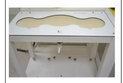
Construction: The shell corresponds to the specifications of the Specific Anthropomorphic Mannequin (SAM) phantom defined in IEEE1528: 2013. It enables the dosimetric evaluation of left and right hand phone usage as well as body mounted usage at the flat phantom region. A cover prevents evaporation of the liquid. Reference markings on the phantom allow the complete setup of all predefined phantom positions and measurement grids by manually teaching three points with the robot.
