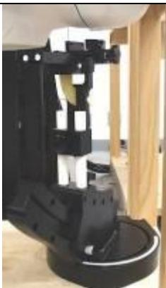
**Construction:** In combination with the Twin SAM Phantom V4.0 or Twin SAM, the Mounting Device (made from POM) enables the rotation of the mounted transmitter in spherical coordinates, whereby the rotation point is the ear opening. The devices can be easily and accurately positioned according to IEC, IEEE, CENELEC, FCC or other specifications. The device holder can be locked at different phantom locations (left head, right head, and flat phantom).
