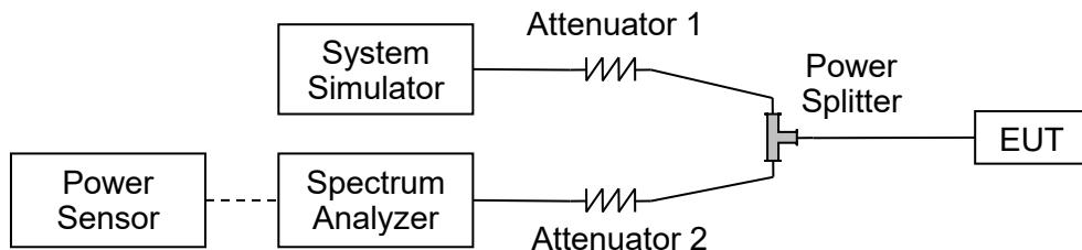
The EUT is coupled to the Spectrum Analyzer (SA) and the System Simulator (SS) with Attenuators through the Power Splitter; the RF load attached to the EUT antenna terminal is 50Ω; the path loss as the factor is calibrated to correct the reading. The EUT is commanded by the SS to operate at the maximum output power. A call is established between the EUT and the SS.
